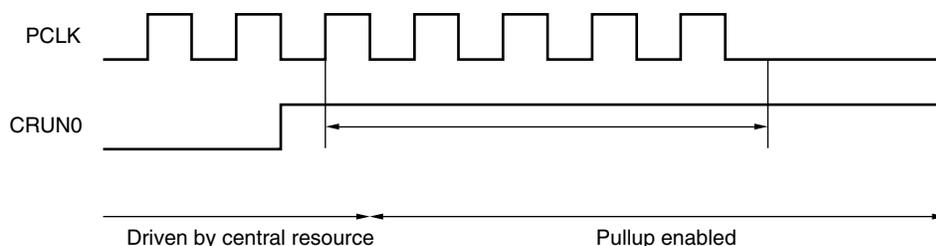
HC asserts CRUN0 asynchronously and it holds CRUN0 asserted until it detects two rising edge of PCLK. After the second clock edge, HC disables its open drain buffer. The central resource drives CRUN0 low at any time after it detects that the line asserted by HC, but not later than on 3<sup>rd</sup> clock. It also must not drive CRUN0 high earlier than on 5<sup>th</sup> clock.
