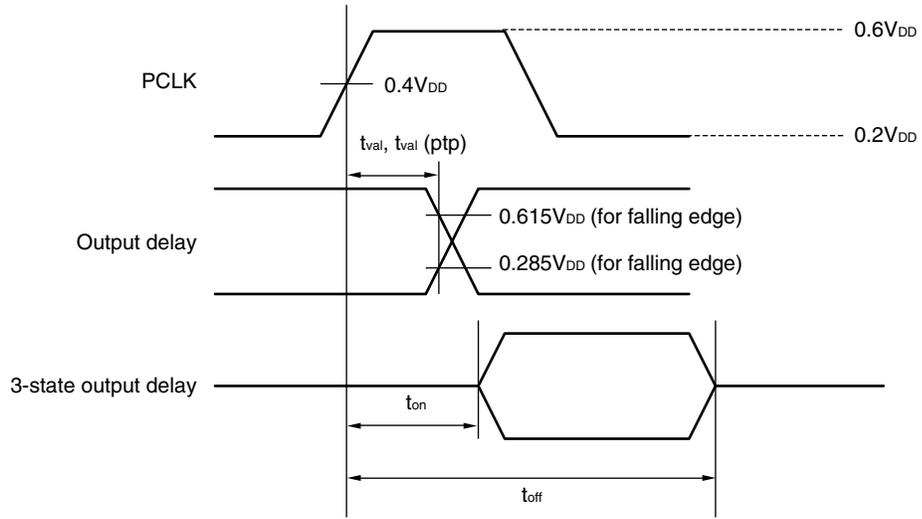
**PCI input timing measurement condition**
