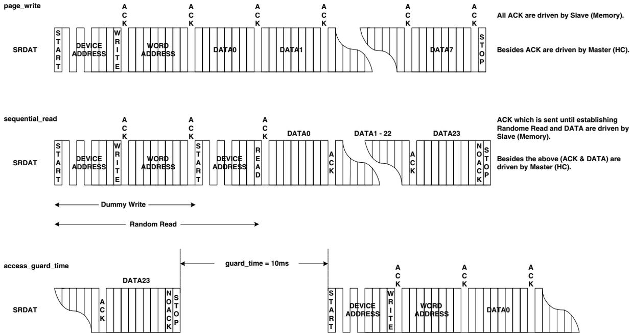
It takes about 2 ms to complete page\_write command and more than 12 ms shall be waited before starting next page\_write or sequential\_read command. On the other hands, It takes about 5 ms to complete sequential\_read command. So, more than 15 ms shall be waited before starting next page\_write or sequential\_read command. And also more than 5 ms shall be waited before reading PCI configuration register after sequential\_read command starts.
