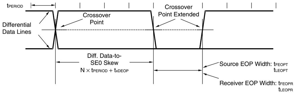
**USB receiver jitter tolerance for low-/full-speed**
