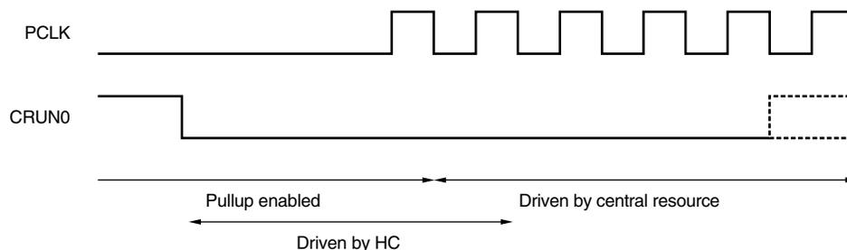
HC may require the PCI clock to complete current internal processes. At that time, HC will assert CRUN0 for two successive clocks after it has been deasserted.
