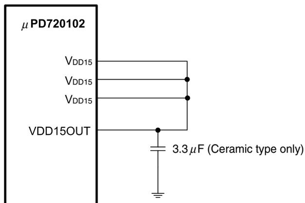
**Caution**  $V_{DD15OUT}$  must be routed to only  $V_{DD15}$  (and  $AV_{DD15}$ ). In case that  $V_{DD15OUT}$  is also used for power supply of other ICs, this may cause unstable operation of the  $\mu$ PD720102.
