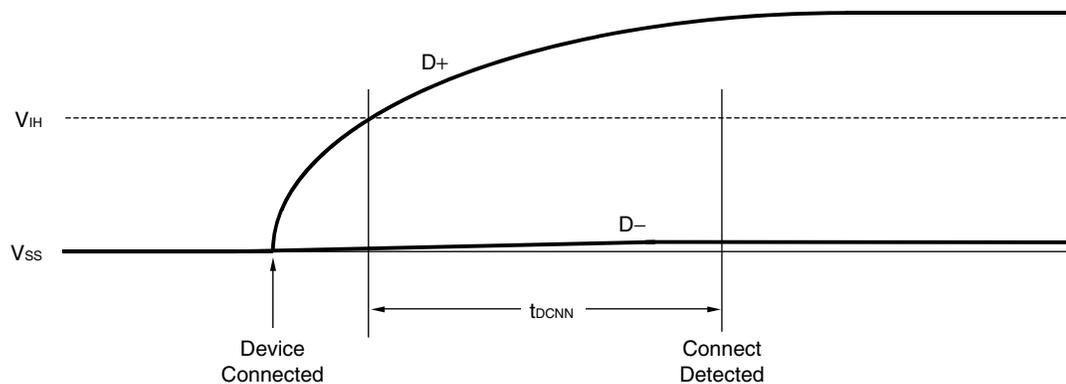
**Low-speed device connect detection**
