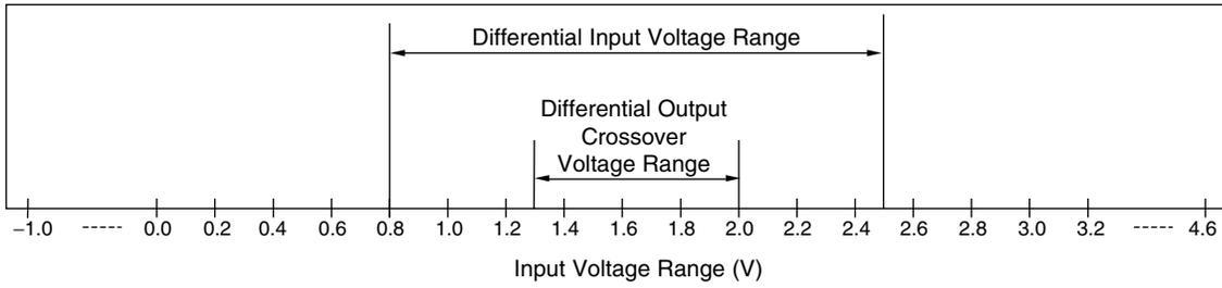
Figure 10-2. Receiver Sensitivity for Transceiver at DP/DM
